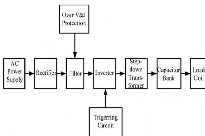
Fig. 1 Block diagram of induction hardening machine
