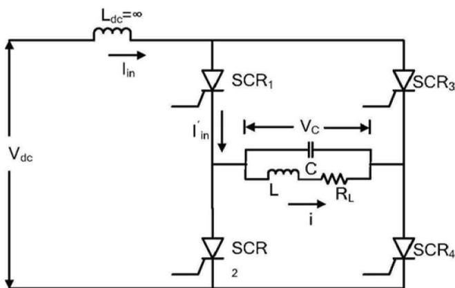
Fig. 3 Current-fed bridge inverter with parallel resonant load
