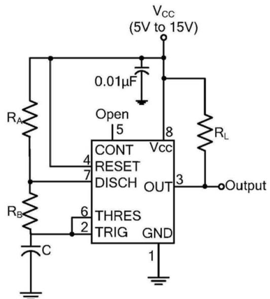
Fig. 4 Starting circuit for inverter triggering circuit
