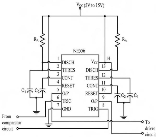
Fig. 5 Dual timer circuit for inverter triggering pulses
