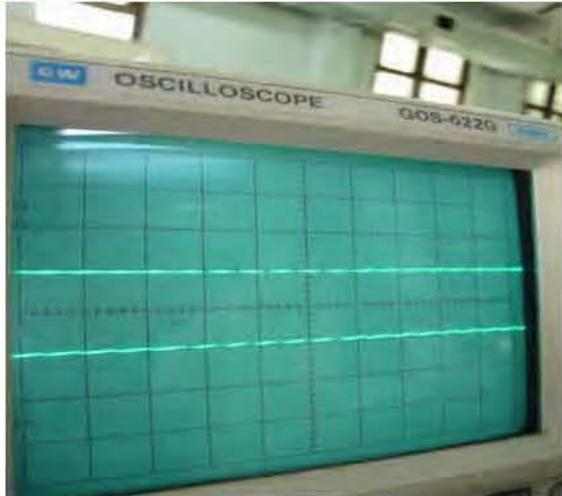
Fig. 9 Test result of SCR input waveform
