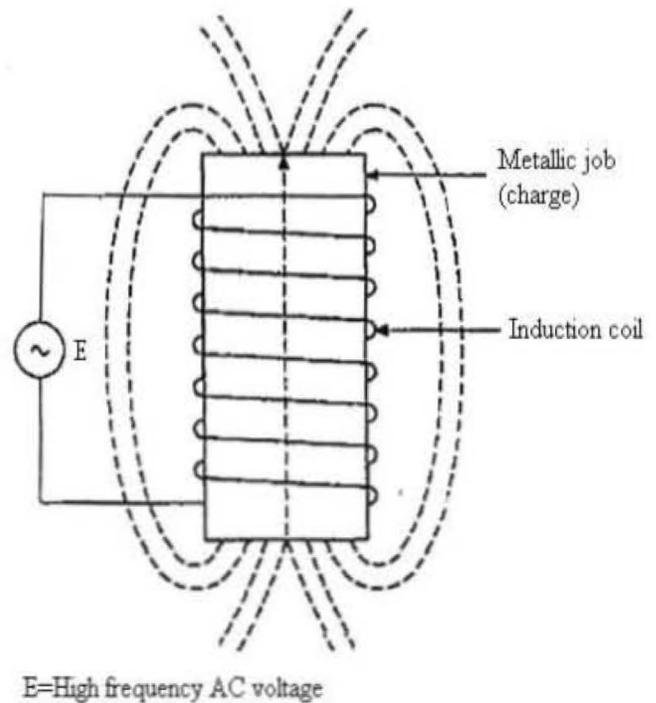
Fig 2 An elementary set-up for the induction hardening process
